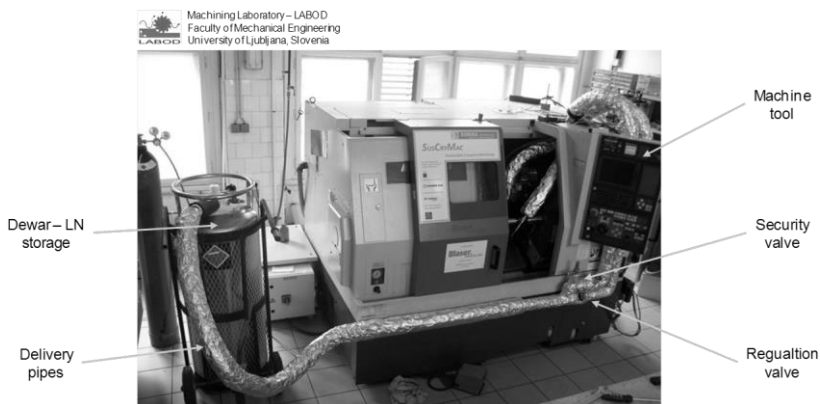
Figure: Cryogenic machining setup on a turret
