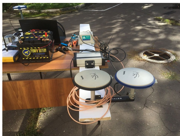
Fig. 6 MAMS pre-flight setup. Two GNSS antennas, GPStation-6 and SPAN-CPT are shown here. Additional Power supply via battery is also presented
