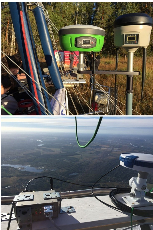
Fig. 10 MAMS-fixed equipment MR-8 and MR-10 are shown at the top and additional GNSS antenna and computation module are shown at the bottom
